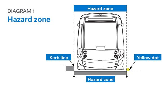
The HAZARD ZONE of the tramway is identified by one or more of the following:
